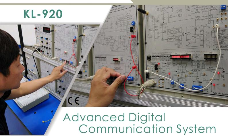
KL-920 is implemented with high speed MCU, DSP and highly flexible FPGA devices, giving students more opportunities to setup and observe digital data signals at each transmission stage.
