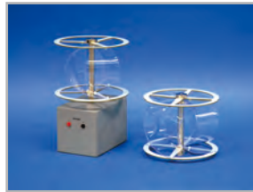
Vertical Axis Wind Turbine
