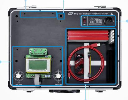
AC power input socket and AC power switch
